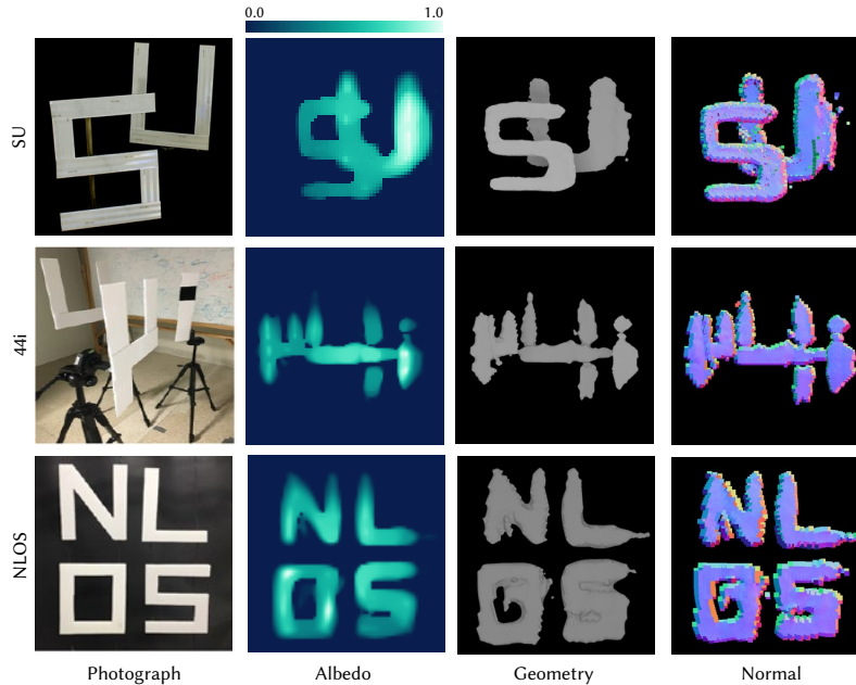
Figure 9: Our inverse rendering results with confocal real scene SU and non-confocal scenes 44i and NLOS. Our approach uses transient measurements to reconstruct surface albedo (second column), geometry (third column), and normals (fourth column), estimating them correctly on multiple isolated objects at different distances.
